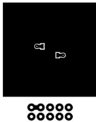
a. 50 °C/W when mounted on a 1 in 2 pad of 2 oz copper, the board designed Q1+Q3 or Q2+Q4.
